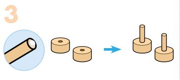
**Step 3**—Add tiny dots of glue to one end of the **paddle handles**. Push the glued ends into the **paddle bases** to make **paddles**. If necessary, lightly tap with a hammer.
