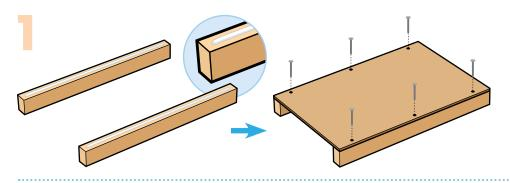
**Step 1**—Lay both side pieces down on the narrow edges. Add thin lines of glue to the top edges. Place the **bottom piece** on top. Make sure outside edges are even. Nail them together.
