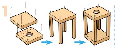
Step 1 - Place the bottom and top pieces flat. Make sure the screw hole by the opening is on top. Start a nail into nail hole in each corner. Glue top of each post under a corner of the bottom piece with corner edges even. Nail them together. Turn the project over. Repeat to attach the top piece.
