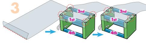
Step 3—Lay the screen flat. Fold one short edge about 1-inch. Turn the project on one side. Hang the 1-inch fold on one of the post. Pull the screen to the 2nd post. Push and LIGHTLY hammer a tack in each corner of the top and bottom pieces. Add a tack to the top and bottom pieces in the middle of the corner tacks.
