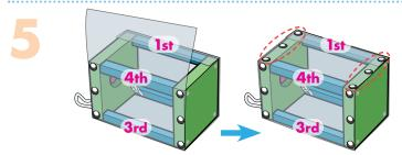
**Step 5—**Turn the project and pull the **screen** tightly to the **1st post**. The end of the screen will overlap the 1-inch fold. Add a tack to each corner then add a tack to the middle of the corner tacks.
