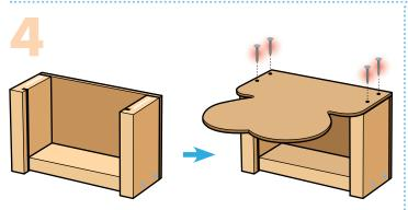
**Step 4**—Turn it up with the **front piece** at the bottom. Add thin lines of glue to the top edge of the **side pieces**. Place the **back piece** on top. Make sure side and bottom edges are even. Using 4 **short nails**, nail it in place.
