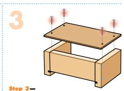
Lay it down with the slots at the bottom. Add thin lines of glue to the top edges. Place the **bottom piece** on top. Make sure all edges are even. Using 4 short nails, nail it in place.
