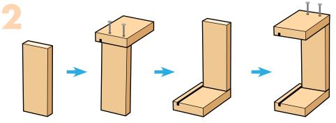
**Step 2—**Stand the **front piece** up. Add a little glue to the top edge. Place one of the **side pieces** on top. Make sure front and bottom edges are even and the slot is not blocked. Nail them together. Turn it over and repeat to attach the other **side piece**.
