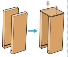
Turn the project on a long, open side. Glue the top piece on top even with the front and side edges so the slots are not covered. Be careful not to put any glue into the slots. Using 4 short nails, nail them together.
