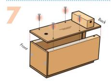
Step 7—Turn both projects over. Glue the bottom piece on top making sure the dowel any glue into the slots. Make sure all edges are even. Using 4 short nails, nail them together to form a trailer.
