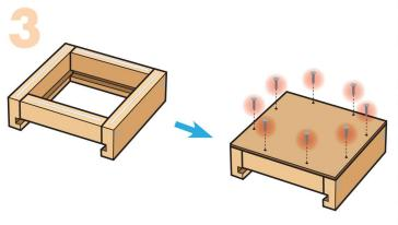
**Step 3—**Turn the project upside down. Add thin lines of glue to the top edge. Place the bottom piece on top. Make sure all edges are even. Using 8 short nails, nail it in place.
