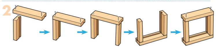
**Step 2—**Stand the **back piece** up. Place one end of the nailed **side** piece on top. Make sure the slots are matching and edges are even. Nail them together.
