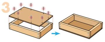
**Step 3**—Lay the project flat. Glue the **bottom piece** on top. Make sure all edges are even. Using 8 **short nails**, nail them together to form a **box**.
