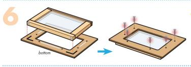
**Step 6**—Lay the **lid** flat with the aiming lines facing up. The edge with the aiming lines is the bottom edge. Add thin lines of glue in between the 2 nail holes on the sides and bottom of the cutout. Using the aiming lines as guide, place the **photo frame** on the **lid**. Hold down the **photo frame** for about a minute so the glue will be sticky. Carefully turn the project over. Using 6 **short nails**, nail them together.
