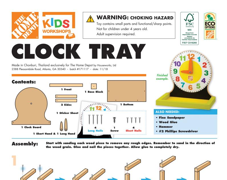
**Step 1**—Lay both **side pieces** down with the nail holes on top. Start 2 long nails. Stand the **front piece** up. Glue one nailed **side piece** on top. Make sure outside edges are even. Nail them together. Turn the project over. Repeat to attach the other **side piece**.
