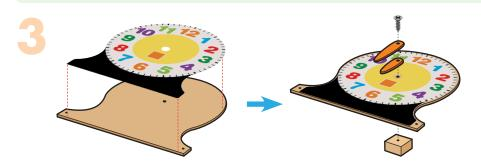
**Step 3**—Lay the **clock board** flat. Carefully add the **sticker**. Match the holes in both **hands** and the **clock board**. Insert a **screw** into the holes. Match the tip of the **screw** to the screw hole in the **base block** and drive the **screw** to attach the **hands** using a **#2 Phillips screwdriver**. Make sure it's tight enough for the **hands** to stay in place but also loose enough for you to adjust.
