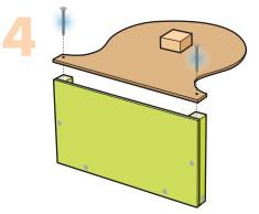
**Step 4**—Stand the **tray** on its front side. Add a little glue to the top of the **side pieces**. Place the **clock board** face side down on top. Make sure sides and bottom edges are even. Using 2 **long nails**, carefully nail them together.
