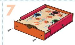
**Step 7**—Attach the **front piece** with 2 **screws**.
