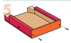
**Step 5—**Attach the **back piece** with 2 **screws**.
