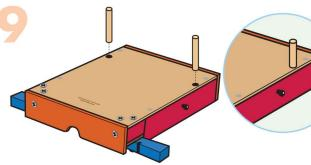
**Step 8**—Add a tiny dot of glue into peg holes of the **flipper bases**. Pick up a **flipper**. The edge with a cutout is the front edge. Aligning the holes, place the **flippers** on top. Push the **large pegs** through the holes to attach them together. Lightly tap with a **hammer** if necessary.
