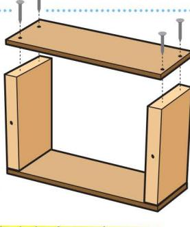
**Step 2** — Stand both **side pieces** up with the holes facing the same direction. Place the **top piece** on top. Ensure the corner edges are even. Nail them together. Turn the **project** over and repeat the step to attach the **bottom piece**.
