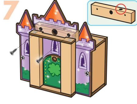
**Step 7** — Attach the **support piece** to the back of the **castle shape** using 2 **screws**. Make sure the vertical peg hole is at the top right.
