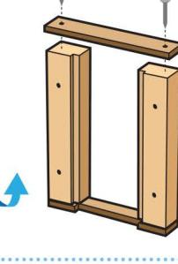
**Step 4** — Stand both **pillars** upright with the holes facing the same direction and the cutouts facing inward.
