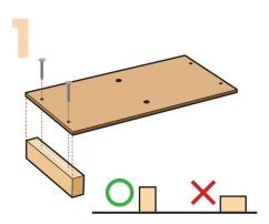
**Step 1**—Place the **end piece** on a narrow, long edge. Add a thin line of glue to the top edge. Place one end of the **bottom piece** on top. Make sure outside edges are even. Nail them together with 2 **nails**.
