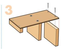
**Step 3**—Stand the **front piece** on a long edge. Add a thin line of glue to the top edge. Place the other end of the **bottom piece** on top. Make sure outside edges are even. Nail them together with 2 **nails**.
