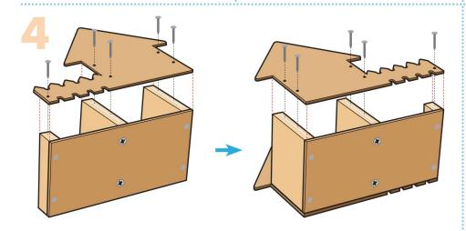
**Step 4—**Turn the project on an open side. Glue a **side piece** on top. Make sure front, back and bottom edges are even. Nail it in place with 5 **nails**. Turn the project over and repeat to attach the other **side piece**.
