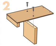
**Step 2**—Stand the **back piece** with the 2 screw holes facing up. Add a thin line of glue in between the 2 screw holes. Place the **bottom piece** on top and align the screw holes in both pieces. Using a #2 Phillips Screwdriver, attach them together with 2 screws.
