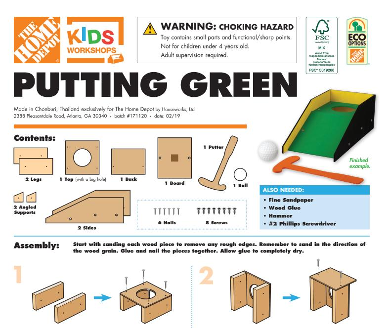
**Step 1**—Stand both **leg pieces** up on long edges. Add a little glue to the top edges. Place the **top piece** on top. Make sure the nail holes are on the **leg pieces** and outside edges are even. Using 4 **nails**, nail them together.
