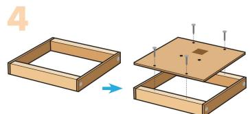
**Step 4**—Lay the project flat. Add thin lines of glue to the top edge of the top and bottom pieces. Place the back on top. Make sure the nail holes are on the top and bottom pieces and all edges are even. Using 4 short nails, nail them together to form a frame.
