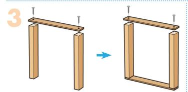
**Step 3**—Stand the **top** and **bottom pieces** up. Glue one of the **side pieces** on top. Make sure outside edges are even. Nail them together with 2 **short nails**. Turn it over and repeat to attach the other **side piece**.
