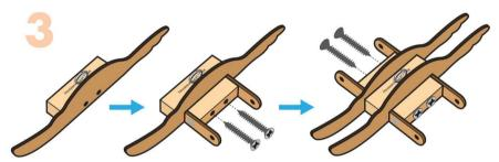
**Step 3** — Place one **body piece** <u>upside down</u> on one side of the **core**, followed by a **connector**, aligning the screw holes in all three pieces.
