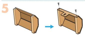
**Step 5**—Add a little glue to the front edge of the **lid side pieces**. Place the **lid front piece** on top with key hole at the bottom. Carefully, attach them together with 2 **short screws** to complete a **lid**.
