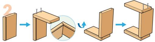
**Step 2—**Stand the **back piece** up. Place the **left side piece** on top. Make sure the slots are matching and back and bottom edges are even. Nail them together. Turn the project over. Repeat to attach the **right side piece**.
