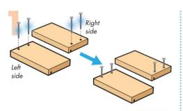
**Step 1**—Lay both side pieces down with slots facing down. Start 4 long nails.
