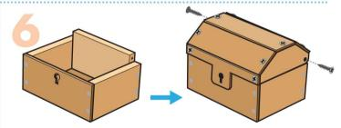
**Step 6**—Fit the **lid** onto the **box**. Make sure screw holes are matching. Attach them together with 2 **long screws**. Don't screw too tightly and make sure the **lid** opens/closes smoothly.
