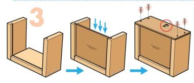
**Step 3**—Turn the project on its back edge. Slide the **bottom piece** into the slots. Add thin lines of glue to the top edge of the **side pieces**. Place the **front piece** on top with key hole at the top edge. Make sure all edges are even. Nail them together with 4 **short nails** to form a **box**. Set aside the **box** until step 6.
