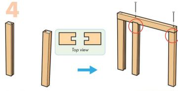
**Step 4** — Stand the **bottom and top frame pieces** up with slots facing in. Add a little glue to the top edges. Fit the notches of the **side piece** to the top edges. Make sure edges are even. Nail them together with 2 nails.
