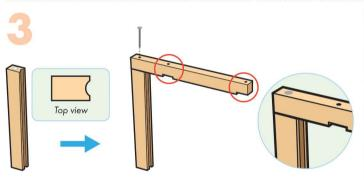
**Step 3 —** Stand the **marker holder** up. Add a little glue to the top edge. Pick up side piece. With the notches facing down, place the bottom corner of the side piece on top of the marker holder. Make sure the groove of the marker holder is facing inward. Make sure edges are even. Nail them together.
