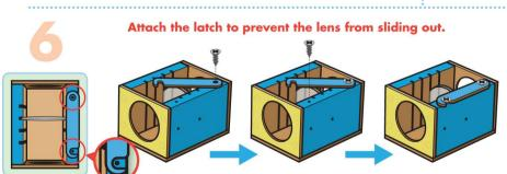
**Step 6**—Place the latch on top of the right side piece with the holes aligned. The cutout at the bottom should be open toward outer edge. First, screw a screw into the top hole using a #2 Phillips Screwdriver. Don't screw too tightly so that the latch can slide.
