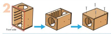
**Step 2—**Lay the project on its front. Make sure the holes in the front edge of the **right side piece** are facing down. Add thin lines of glue to the top edge of the side pieces. Place the back piece on top. Make sure all edges are even. Nail them together to form an observation box.
