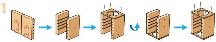
**Step 1**—Stand both side pieces up with the holes in side edges located toward bottom. Turn them inward so slots are facing in. Add thin lines of glue to the top edges.
