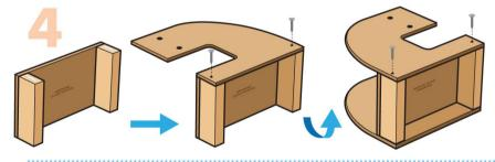
**Step 4—**Turn the project on one side. Add a little glue to the top edge of the supports. Pick up one frame. The straight edge with 2 holes is the bottom edge. Place the bottom edge of the frame on top of the project. Make sure front, back and bottom edges are even. Nail them together. Turn the project over and repeat to glue and nail the other frame.
