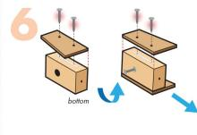
**Step 6**—Turn the **console** on one side. Pick up one **side panel**. The wider edge is the bottom. Glue the **side panel** on top. The **side panel** hangs over the side with the big hole. Make sure outside edges are even. Nail them together with 2 **short nails**. Turn the **console** over and repeat to attach the other **side panel**.
