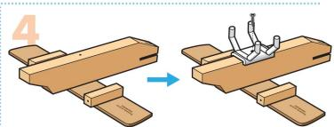
**Step 4**—Turn the project over. Align the hole in the **strut** to the hole in the bottom of the **body**. Using a **long screw**, attach the **strut** to the **body**.
