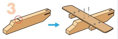
**Step 3**—Place the **body** with a line on top. Using the line as a guide, center and glue the **wing** on top. Make sure **motors** are under the **wing** and sticking out toward the front. Using 2 nails, nail the wing to the body.
