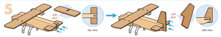
**Step 5**—Turn the project over and rotate it to the back edge with horizontal and vertical slots. Pick up the **rear wing**. The long straight edge is the front. Add a little glue to the center of the front edge. Push it into the horizontal slot and align the cutout with the vertical slot. Add a little glue to the notch of the tail fin. Push it into the vertical slot. Before moving on to next steps, wait about 5 minutes for the glue to get tacky.
