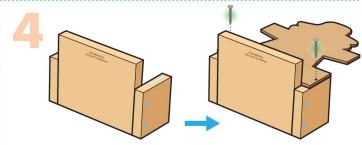
**Step 4**—Turn the project on the front edge. Glue the **scarecrow** to the **side pieces**. Make sure top and side edges are even. Nail it in place with 2 **medium nails**.
