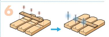
**Step 6**—Lay the 3 **pickets** down with cutout for the **rail** facing up. Add a little glue to the cutouts. Place the **rail** in the cutouts. Make sure side edges are even and the **picket** in the middle is centered. Carefully, nail them together with 3 **short nails** to form a **picket fence**.
