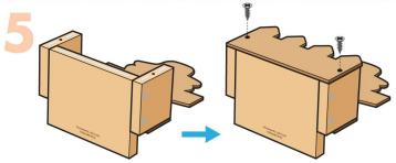
**Step 5—**Turn the project over. Glue the **front fence** to the front edge. Align the screw holes in the **front fence** and **side pieces**. Attach them together with 2 **screws** using a **#2 Phillips Screwdriver**. Set aside the project until Step 7.
