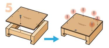
**Step 5** — Turn the project upside down. Apply thin lines of glue along the top edge.
