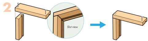
**Step 2** — Stand the **back piece** up. Place one end of a started **side piece** on top. Make sure the slots are matching and the edges are even. Nail them together.
