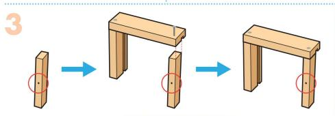
**Step 3** — Stand the **front piece** up. The edge with a screw hole is the bottom.
