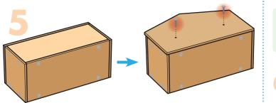
**Step 5**—Lay the project on one side. Glue the **firehouse front** even with side and bottom edges. The **firehouse front** extends above the top edge. Using 2 **short nails**, nail it in place.
