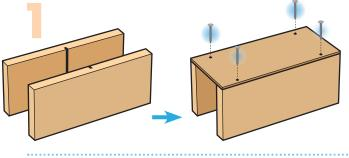
**Step 1**—Stand the **front** and **back pieces** on the long edges with screw holes down and the slots facing in. Glue the **bottom piece** on top. Make sure all edges are even. Using 4 **long nails**, nail it in place.
