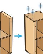
**Step 3**—Stand the project on one end. Glue one **end piece** on top. Make sure all edges are even and the nail holes are on the **front** and **back pieces**. Using 4 **long nails**, nail it in place. Turn the project over and repeat to attach the other **end piece**.
