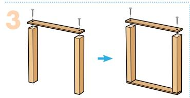
**Step 3**—Stand the **top** and **bottom pieces** up. Glue one of the **side pieces** on top. Make sure outside edges are even. Nail them together with 2 **short nails**. Turn it over and repeat to attach the other **side piece**.
