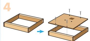
**Step 4—**Lay the project flat. Add thin lines of glue to the top edge of the top and bottom pieces. Place the back on top. Make sure the nail holes are on the top and bottom pieces and all edges are even. Using 4 short nails, nail them together to form a frame.
