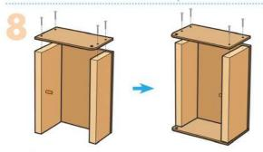
**Step 8**—Stand the project up. Place the **top piece** on top. Make sure edges are even and there is a space for the **hinge** under the rounded corner. Nail them together with 4 **nails**. Turn the project over and repeat to attach the **bottom piece** to form a **locker**.
