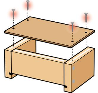
**4** **Step 4**—Turn it up with the front piece at the bottom. Add thin lines of glue to the top edge of the side pieces. Place the back piece on top. Make sure side and bottom edges are even. Using 4 short nails, nail it in place. Turn the project right side up. Slide the lid into the slots.
