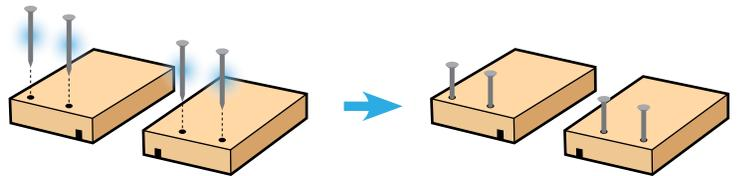
**2** **Step 2**—Stand the front piece up. Add a little glue to the top edge. Place one of the side pieces on top. Make sure front and bottom edges are even and the slot is not blocked. Nail them together. Turn it over and repeat to attach the other side piece.
