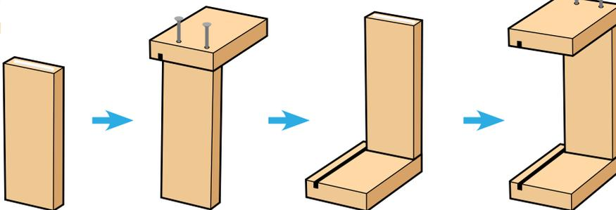
**3** **Step 3**—Lay it down with the slots at the bottom. Add thin lines of glue to the top edges. Place the bottom piece on top. Make sure all edges are even. Using 4 short nails, nail it in place.
