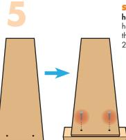
Step 5-Lay the lid flat. Glue the handle under the edge with the nail holes. Make sure the lid is centered on the **handle** and edges are even. Using 2 short nails, nail them together.
