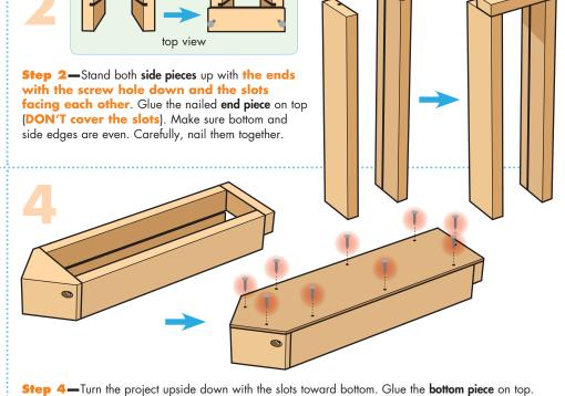
Make sure all edges are even. Using 9 short nails, nail it in place.
