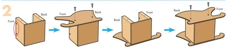
**Step 2—**Turn the project on an open side. Match the holes in one **sled side piece** to the holes in the **front** and **back pieces**. Make sure the front edge of the **sled side piece** is on the **front piece**. Glue this **sled side piece** and attach securely with 2 **screws**. Turn the project over and repeat to attach the other **side piece** to form a **sled**.
