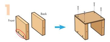
**5tep 1** — Stand both **front** and **back pieces** on long edges. Make sure the holes for the **string** in the **front piece** are at bottom. Glue the **bottom piece** on top. Make sure the nail holes are on the **front** and **back pieces**. Make sure outside edges are even. Using 4 **nails**, nail them together.
